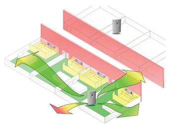
Hallway Installed AP Extensive Planning Disruptive Installation Expensive cable pull Guest Room Installed AP Rapid Deployment Uses Existing CAT5/6 Cabling Integrated Controller
